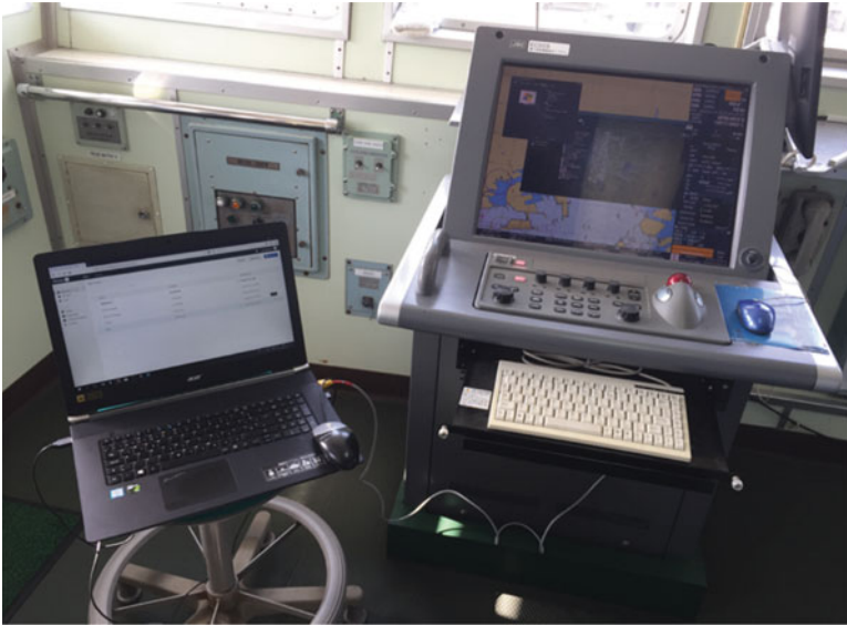
Figure 3. Testing setup for computational vulnerability scanning of ECDIS.
